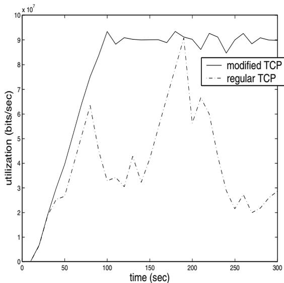
Fig. 4. Link Utilization averaged over 10 sec. intervals.
