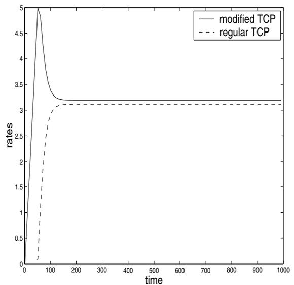
Fig. 2. TCP Friendliness of the modified TCP congestion controller.
