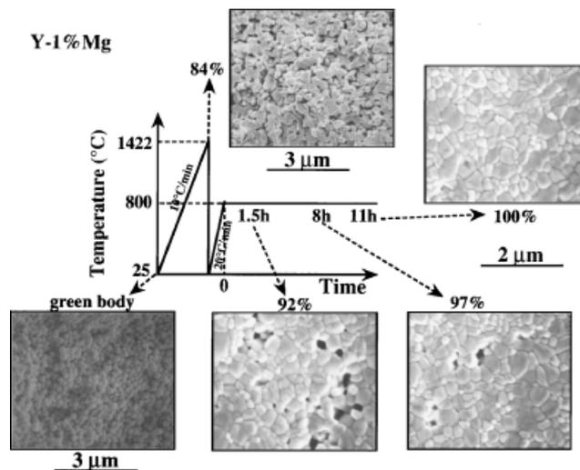
Fig. 1. Summary of two-step sintering experiment using  $\text{Y}_2\text{O}_3$  (with 1%  $\text{Mg}^{2+}$ ) starting with spherical powders of a particle size 200 nm. No grain growth (grain size 390 nm) was observed in the second step.
