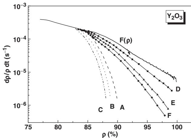
**Fig. 5.** Normalized densification rate of  $Y_2O_3$  samples in second-step sintering. Curves are shifted vertically for easy comparison with the universal density function  $F(\rho)$ . Same notation as in Fig. 3. No grain growth was observed but densification was incomplete in A, 1310°, 1000°C—10 h; B, 1250°, 1000°C—10 h; and C, 1250°, 950°C—10 h. Grain growth was observed in D, 1310°, 1300°C—10 h; E, 1310°, 1250°C—10 h; and F, 1310°, 1200°C—10 h.
