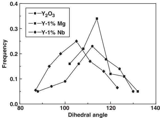
Fig. 2. Dihedral angles of undoped and doped  $Y_2O_3$ .
