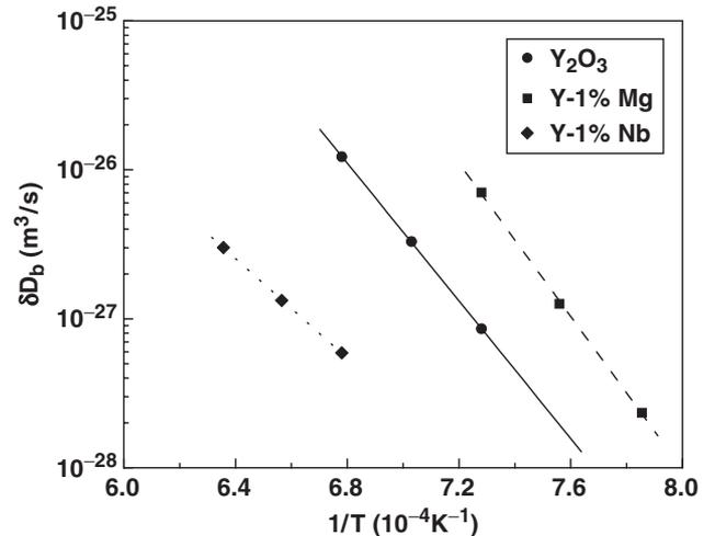
Fig. 4. Estimated grain boundary diffusivity against reciprocal temperature.
