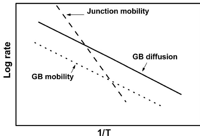
**Fig. 10.** Schematic Arrhenius plot for grain-boundary diffusion, mobility of pore/grain-boundary junction or four-grain junction, and intrinsic mobility of grain boundary (without drag) which is parallel to grain-boundary diffusion.
