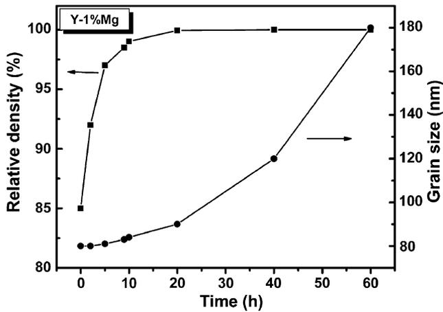
Fig. 7. Density and grain size of  $\text{Y}_2\text{O}_3$  (with 1%  $\text{Mg}^{2+}$ ) sintered in the second step at  $1000^\circ\text{C}$  for 60 h. Sample previously preheated to  $1120^\circ\text{C}$  ( $T_1$ ) without holding.
