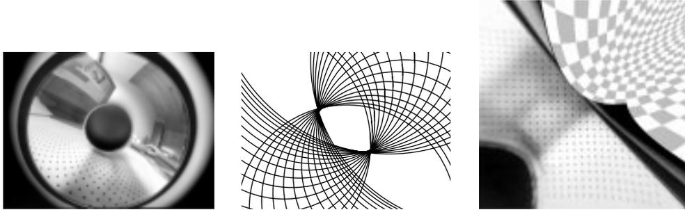
Figure 10: Left: Original image taken by a folded catadioptric camera. Middle: Circles fitted to points captured from the grid. Notice that the lines of the grid are parallel and thus their projections, circles, intersect in the image at vanishing points. Using these line images we perform a calibration and rectification, i.e. finding the normal of the plane containing the grid. Right: A reprojection to a plane parallel to the grid.
