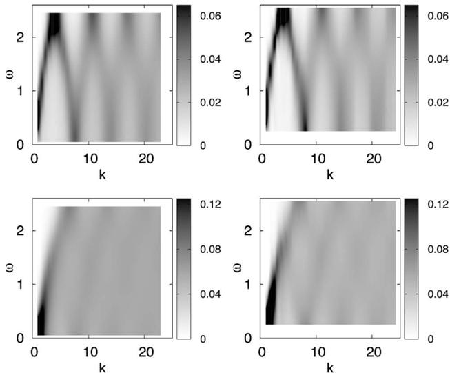
FIG. 9. Dispersion relation at two different compressions for  $N=1024$  monodisperse spheres in 3D. Left panels:  $\Delta\phi=1\times 10^{-6}$ . Right panels:  $\Delta\phi=1\times 10^{-1}$ . Top and bottom panels correspond to longitudinal and transverse modes, respectively. Darker shading corresponds to larger amplitude in  $f_{L,T}$ . The maxima of the transverse amplitudes are typically a factor of 5 larger than for the longitudinal data. The bars to the right indicate the amplitude scale.
