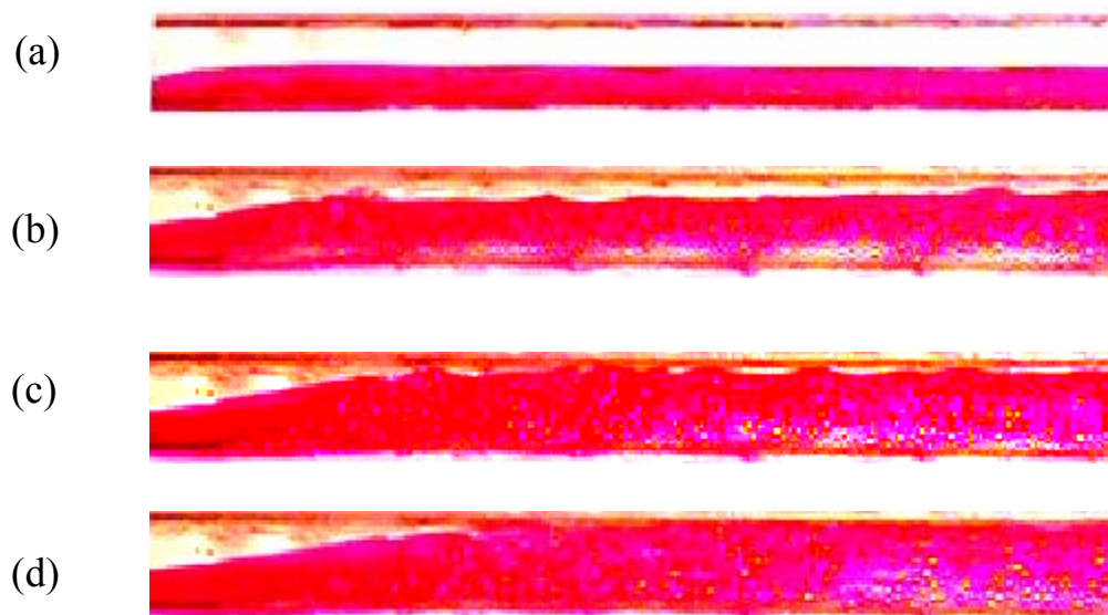
Fig.16: The spread of the dye in the flow-through stirrer at times t=0 (a, inactive stirrer), t=T/2 (b), t=T (c) and t=3T/2 (d). A potential difference of \Delta V=2.0V is imposed between the active electrodes. Different pairs of electrodes are alternately engaged with a period T=4s . The average fluid velocity is 5mm/s , and the net flow rate is 2ml/s .
