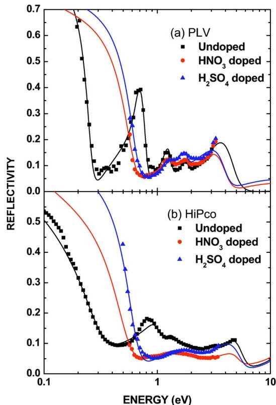
FIG. 4. (Color online) The reflectivity and Drude-Lorentz fits for undoped, HNO<sub>3</sub>-doped, and H<sub>2</sub>SO<sub>4</sub>-doped PLV (a) and HiPco (b) buckypapers. Two systematic effects are observed: a blueshift of the reflectivity minimum (increasing Drude plasma frequency) and decreased intensity of the peaks at higher energy (quenching interband transitions by shifting  $E_F$ ). See Table I for model fit parameters (solid curves).
