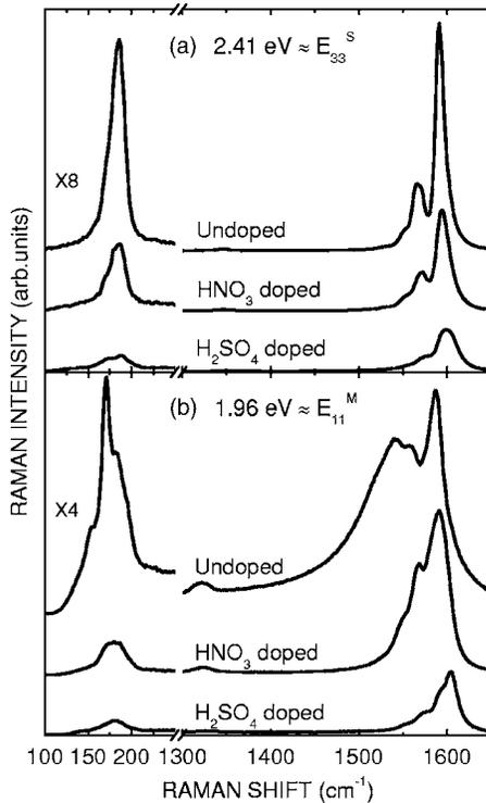
FIG. 5. The Raman spectra of undoped,  $\text{HNO}_3$ -doped, and  $\text{H}_2\text{SO}_4$ -doped PLV buckypapers using (a) 2.41 eV and (b) 1.96 eV laser excitation. The RBM bands are magnified for clarity. Raman intensities decrease upon doping, more dramatically for sulfuric acid.
