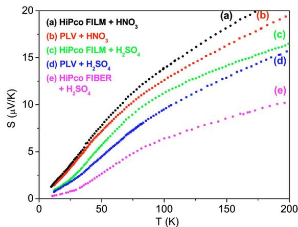
FIG. 3. (Color online) The doping effect on thermopower. For undoped and air-exposed SWNT  $S(T)$  increases monotonically to  $60\text{--}80\text{ }\mu\text{V/K}$  at  $300\text{ K}$  (not shown). Doping reduces the amplitude at all  $T$  and introduces an inflection point at characteristic temperatures in the range  $20\text{--}50\text{ K}$  for different samples. Both effects are most apparent in the  $\text{H}_2\text{SO}_4$ -doped HiPco fiber.
