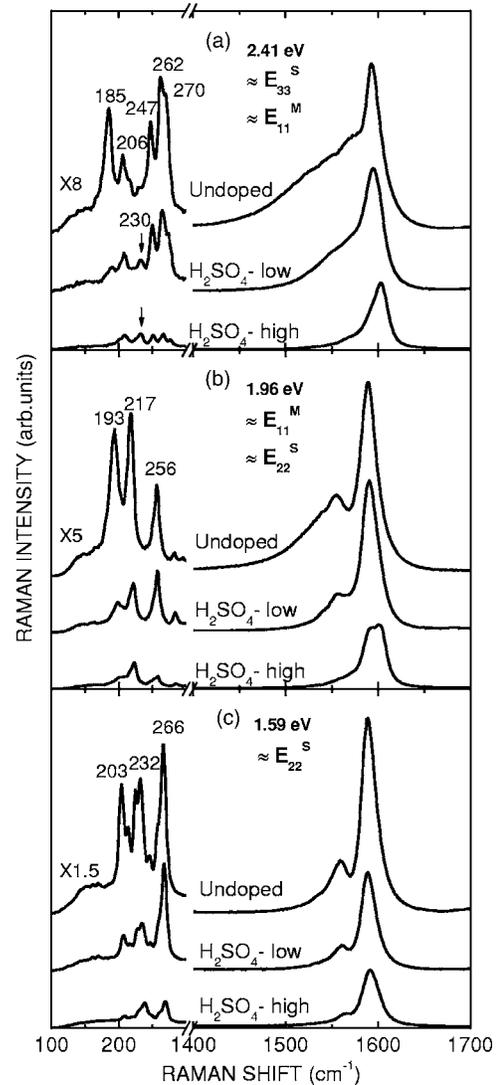
FIG. 6. The Raman spectra of HiPco fibers using (a) 2.41 eV, (b) 1.96 eV, and (c) 1.59 eV laser excitation. The RBM bands are magnified for clarity. “Low” and “high” concentrations of  $\text{H}_2\text{SO}_4$  were obtained using different coagulation baths in the spinning process. The loss of resonance upon doping is similar to PLV (Fig. 5). See Table II for estimated  $E_F$  shifts associated with loss of Raman resonance.
