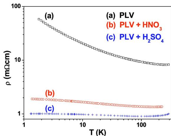
FIG. 2. (Color online) The doping effect on resistivity and its temperature dependence. Doping reduces  $\rho(300\text{ K})$ , approximately twice as much for sulfuric than nitric acid. The temperature dependence becomes weaker after doping, more dramatically so for sulfuric than nitric acid.
