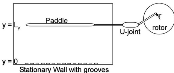
FIG. 7. A schematic of the experimental setup that applied oscillatory planar shear to the bubble rafts. The  $U$  joint highlighted in the figure is used to convert the rotary motion of the driving motor into oscillatory planar shear.
