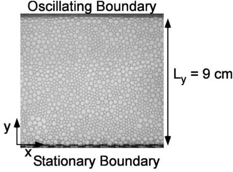
FIG. 1. A typical snapshot of the 2D bubble raft used in experiments with packing fraction  $\phi \approx 0.86$  and  $N \approx 3700$  bubbles. The bubble raft is composed of a bidisperse distribution of bubble sizes: a 4 to 1 ratio of  $2.5 \pm 0.3$ -mm- to  $5.3 \pm 0.5$ -mm-diameter bubbles.
