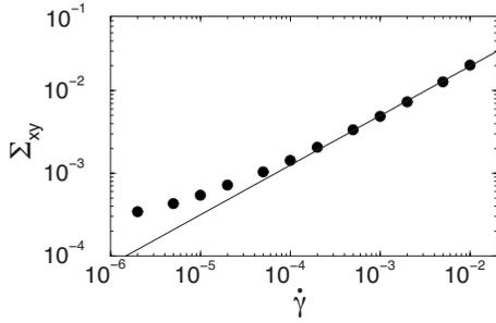
FIG. 6. Average shear stress  $\Sigma_{xy}$  plotted versus the applied shear rate  $\dot{\gamma}$  for a system with  $\phi=0.86$  and  $b^*=2$  undergoing steady planar shear flow in 2D simulations of the bubble model. The cross-over shear rate at which the system transitions from quasistatic to power-law behavior is  $\dot{\gamma}_c \approx 10^{-4}$ .
