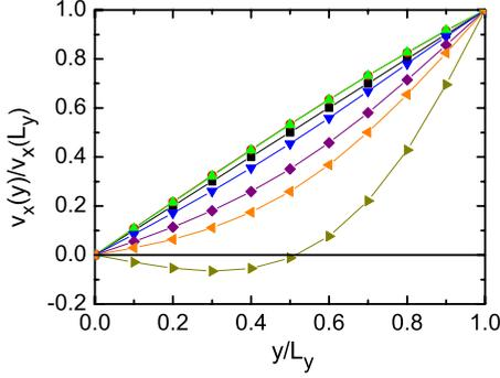
FIG. 3. (Color online) Normalized horizontal velocity profiles  $v_x(y)/v_x(L_y)$  at  $t=0$  for a viscoelastic material with  $\beta = G\rho L_y^2/\eta^2 = 1$  obtained from solutions to Eq. (1) as a function of the driving frequency  $\omega$ . We show  $\omega/\omega_{nl}=0.1$  (squares), 1.1 (circles), 2.1 (upward triangles), 4.1 (downward triangles), 6.1 (diamonds), 8 (left triangles), and 20 (right triangles).  $\omega_{nl}$  corresponds to  $\omega_{nl}^l = \omega_{nl}^s$ .
