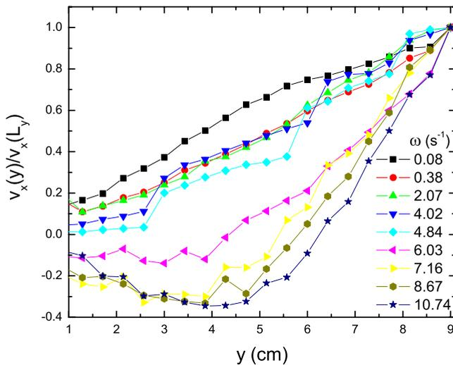
FIG. 9. (Color online) The normalized average horizontal velocity  $v_x(y)/v_x(L_y)$  (averaged over times when the boundary velocity is maximum) as a function of distance  $y$  from the stationary bottom wall for several driving frequencies  $\omega$  in the bubble raft experiments. At frequencies  $\omega < \omega_d \approx 4.0 \text{ s}^{-1}$ , the profiles are roughly linear, while above this characteristic frequency, liquidlike nonlinear profiles are observed.
