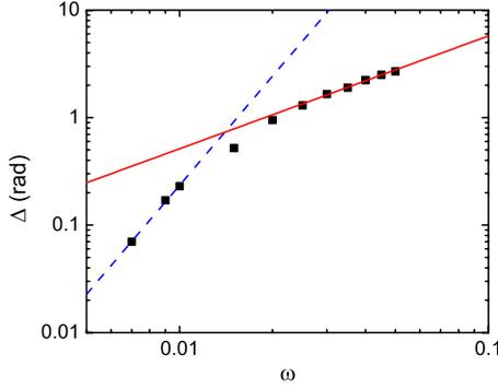
FIG. 12. (Color online) Total phase difference  $\Delta$  plotted as a function of the driving frequency  $\omega$  for the bubble model simulations at  $\phi=0.86$  and  $b^*=2$ . From the intersection of the solid red and dashed blue lines with slopes 1 and 3, respectively, we estimate  $\omega_p \approx 0.015$ .
