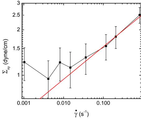
FIG. 8. (Color online) Shear stress  $\Sigma_{xy}$  versus the applied shear rate  $\dot{\gamma}$  for the same bubble raft system described in Fig. 1 undergoing steady planar shear. We estimate the crossover frequency  $\dot{\gamma}_c \approx 0.065 \text{ s}^{-1}$  above which the system transitions from the quasi-static to the power-law flow regime.
