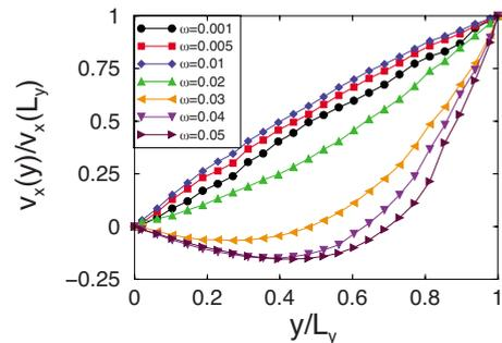
FIG. 11. (Color online) The normalized average velocity  $v_x(y)/v_x(L_y)$  (averaged over times when the boundary velocity is maximum) as a function of distance  $y$  from the stationary wall plotted for several driving frequencies  $\omega$  in the bubble model simulations. For  $\omega \geq \omega_d \approx 0.02$ , the velocity profiles display liquidlike nonlinear decay.
