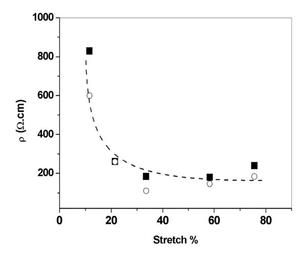
**Figure 2:** 4-probe electrical resistivity at room temperature vs. stretch ratio for composite nanotube fibers. The experiments have been conducted on two series of samples (black squares, open circles). Accurate cross-sectional areas were obtained from SEM image analysis. The resistivity decreases with stretch ratio by a factor between 3 and 4 for the two set of data. The absolute value is intermediate between all-SWNT fibers and polymer composites. The dashed line is a guide to the eye.
