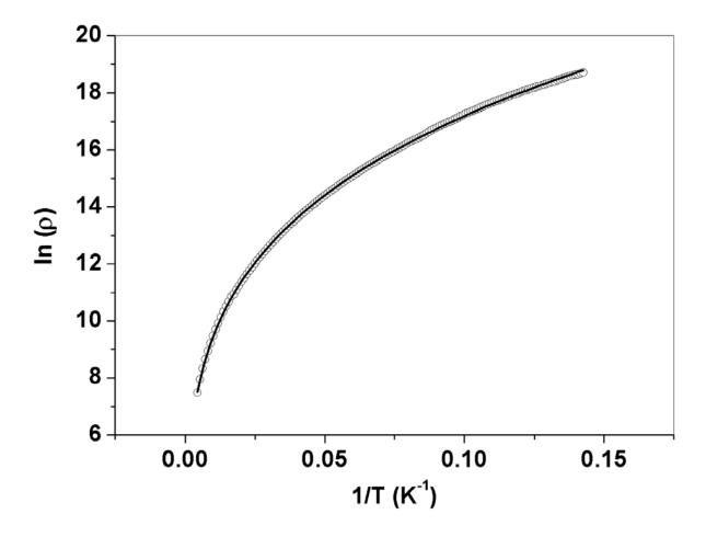
**Figure 6:** Fit using a generic strong localization model (solid curve) to the data from a PVA/SWNT composite 80% stretched sample (solid squares). The fit is excellent at all temperatures but the parameters are unphysical for either phonon-assisted or Coulomb gap VRH (see text).
