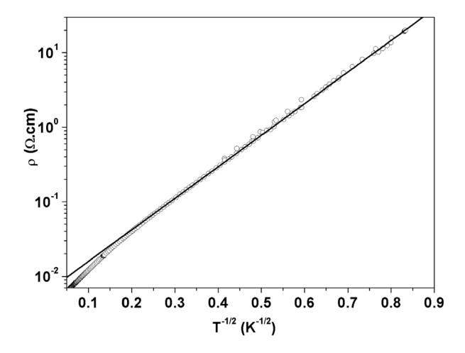
**Figure 5:** Fit to a model of strong localization (solid curve) to the data from annealed 76% stretch sample (solid squares). The fit is excellent at low temperatures T < 25K and over 3 decades of  $\rho$ . The characteristic temperature in the factor  $\exp(T_0/T)^{1/2}$  is 95K, or  $\sim$  8 meV, which we associate with a Coulomb gap (see text).
