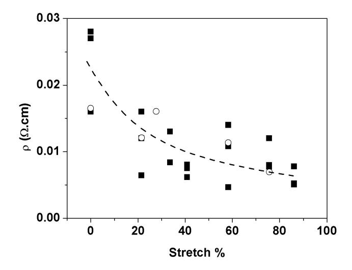
**Figure 3:** 4-probe electrical resistivity at room temperature vs. stretch ratio for 2 sets of annealed nanotube fibers. Cross-sections were determined from optical microscopy and are therefore less accurate than in Figure 2. The trend of decreasing  $\rho$  with increasing stretch % is less apparent than in Figure 2. The resistivity decreases dramatically upon removal of the non-conducting PVA.
