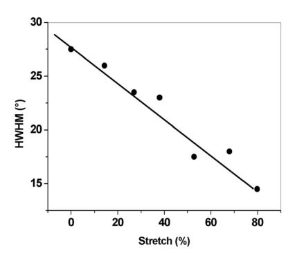
**Figure 1:** Gaussian half width at half maximum (HWHM) vs. stretch ratio for PVA/SWNT composite nanotube fibers. The initial alignment (stretch % = 0) results from extrusional flow during spinning. This improves due to extensional flow under tension.
