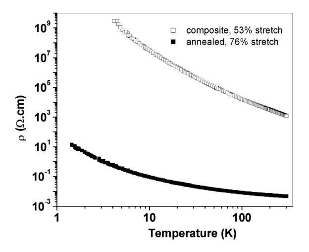
**Figure 4:** Resistivity vs. temperature for composite (53% stretch) and annealed (76% stretch) nanotube fibers (note log-log scale). Note that  $\rho(T)$  for the composite fiber is more strongly divergent as  $T \rightarrow 0$  as compared to the annealed one.
