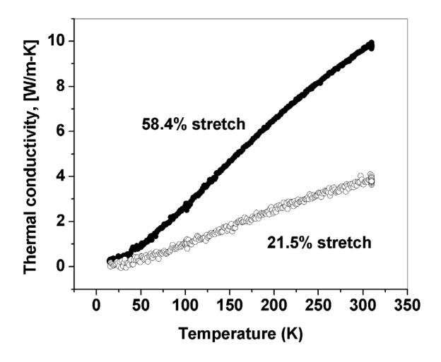
**Figure 7:** Thermal conductivity vs. temperature for annealed nanotube fibers which have been stretch-aligned to 21% (lower curve) and 58% (upper curve). Additional alignment of the latter yields a fator  $\sim$ 2 further enhancement of  $\kappa$ . The temperature dependence is dominated by that of the lattice specific heat, as is generally observed.
