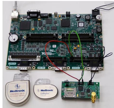
**Figure 3: Closed-loop experimental setup with heart model on the FPGA board and pacemaker implemented on the FireFly sensor node. Medtronic cardiac defibrillator and pacemaker models are shown for reference.**
