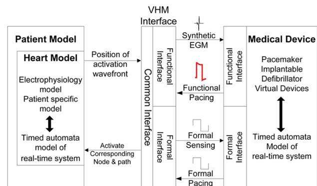
Figure 1: Structure of the heart model platform
