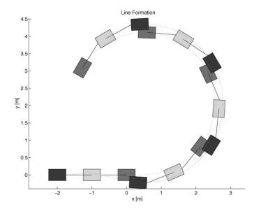
Fig. 7. Robot paths for the cascade formation.
