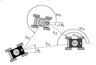
Fig. 5. Three mobile robots using separation-bearing controllers.
