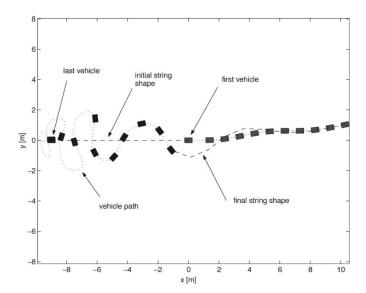
Fig. 3. String of 10 vehicles tracking a sinusoidal trajectory.
