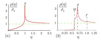
FIG. 3 (color online). Density of states as a function of  $\eta = \omega/\omega^*$  for (a) the square and (b) kagome lattices, showing their constant value when k' = 0 (dashed green line) and van Hove singularities, from the saddle at S and minima at M and  $\Gamma$ , whose frequencies all scale as  $\omega^* \propto \sqrt{k'}$  when k' > 0.
