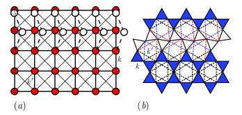
FIG. 1 (color online). (a) Square and (b) kagome lattices with NN springs of spring constant k and NNN springs of spring constant k'. White circles in (a) and white triangles in (b) show a zero-energy distortion.
