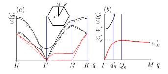
FIG. 4 (color online). (a) Phonon dispersion along symmetry directions. The dotted lines are for k'=0 and the solid lines are for k'=0.02. The isostatic and quasi-isostatic branches are in red. (b) shows isostatic and shear modes along  $\Gamma M$  and indicates characteristic frequencies and wave-numbers.
