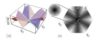
FIG. 5 (color online). (a) Plot of iso mode at k' = 0. (b) density plot of iso mode at k' = 0.02k. Inset: circular symmetry at origin.
