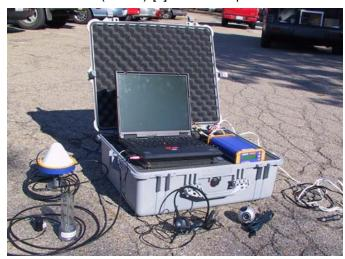
**Figure 2.** Portable multi-hop mobile test-bed with DGPS receiver and onboard computer
