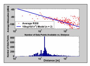
**Figure 5.** Total Average Measured Signal Attenuation and Free Space Propagation Model vs. Distance
