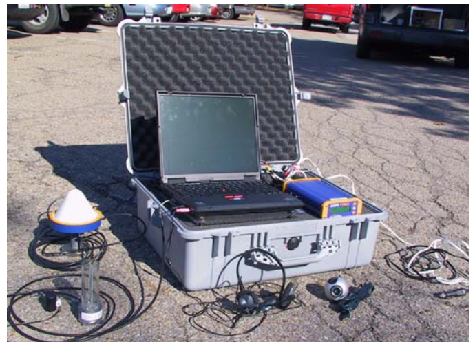
Figure 2. Portable multi-hop mobile test-bed with DGPS receiver and onboard computer
