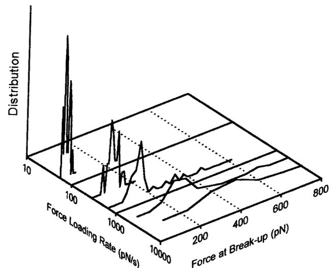
FIGURE 8 Curves showing the distribution of force at breakup for five different loading rates. The number of trials included at each different rate were: 25 at both  $57 \text{ pN s}^{-1}$  and  $285 \text{ pN s}^{-1}$ , 40 at  $650 \text{ pN s}^{-1}$ , 23 at  $1800 \text{ pN s}^{-1}$ , and 66 at  $3600 \text{ pN s}^{-1}$ . Note that the distributions broaden with increasing loading rate.
