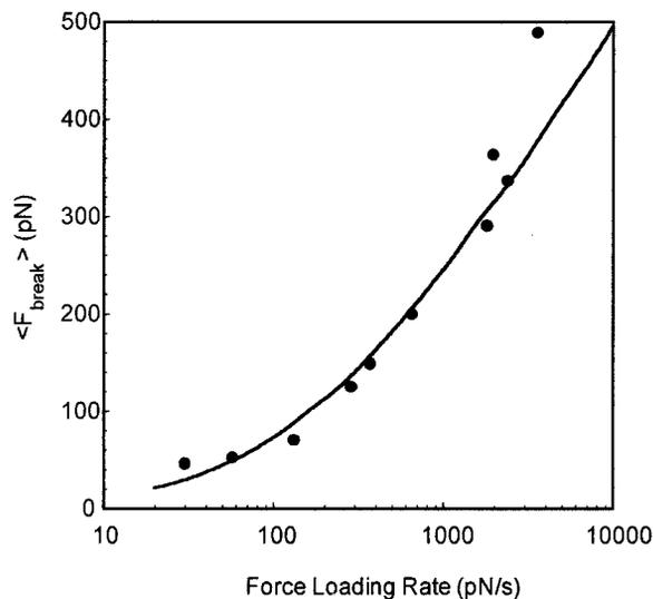
FIGURE 11 Data from Fig. 9 with the superimposed *solid line* indicating  $\langle F_{\text{break}} \rangle$  versus  $\ln r_f$  computed from Eq. 12 using the best fit Bell model parameters  $k_r^o = 0.82 \text{ s}^{-1}$  and  $r_o = 0.034 \text{ nm}$ .
