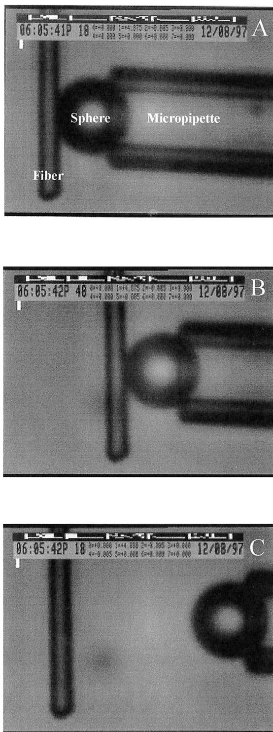
FIGURE 1 A sequence of video frames from an adhesive event. In frame A, the bead and fiber are apposed, with the fiber given a small negative displacement with respect to its rest position (frame C). In frame B, the micropipette is retracted and a bond between bead and fiber leads to positive deflection of the fiber. Immediately after this frame, the bond dissociated. Frame C shows the bead and fiber in their final rest positions.
