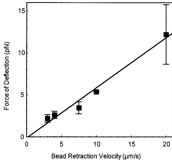
FIGURE 6 Bead-retraction-induced hydrodynamic force on fibers versus bead retraction velocity.
