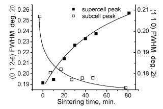
**Fig. 6.** Supercell (filled dots) and subcell (open dots) XRD peak width versus sintering time for LiNb<sub>0.6</sub>Ti<sub>0.5</sub>O<sub>3</sub>–V<sub>2</sub>O<sub>5</sub> composites.
