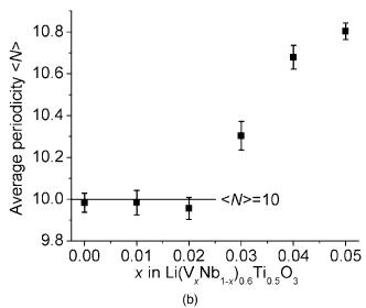
**Fig. 1.** Lattice parameters of  $\text{Li}(\text{Nb}_{1-x}V_x)_{0.6}\text{Ti}_{0.5}\text{O}_3$  powders versus doping level (x): (a) a (filled dots) and c (open dots) lattice parameters calculated for N=10 M-phase cell, (b) M-phase superstructure periodicity  $\langle N \rangle$  (see text).
