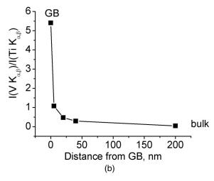
**Fig. 5.** Evidence for V-rich liquid phase in  $\text{LiNb}_{0.6}\text{Ti}_{0.5}\text{O}_3-\text{V}_2\text{O}_5$  composites: (a) grain boundary layer observed in a sample annealed for 30 min; (b) intensity ratio of V and Ti EDX signal versus distance from grain boundary layer.
