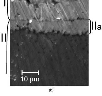
**Fig. 4.** Metallization compatibility of x=0.02 sample (a) powder XRD pattern of  $V_2O_5$ -doped M-phase–Ag powder composite before (black line) and after (gray line) annealing at 900°C; stars denote Ag peaks; (b) secondary-electron SEM image of a cross section of x=0.02 sample metallized as a green body and then annealed at 900°C, where I is the metallization layer, II is the ceramic layer, and IIa is the top part of the ceramic layer (see text).
