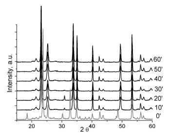
**Fig. 7.** X-ray diffraction patterns of reactively sintered samples as a function of annealing time. Gray line represents the pattern of initial mixture of  $\text{Li}_2\text{TiO}_3$ ,  $\text{LiNbO}_3$ ,  $\text{TiO}_2$ , and  $\text{V}_2\text{O}_5$ .
