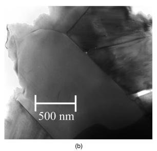
**Fig. 8.** Microstructure of reactively sintered samples: (a) liquid-phase associated features (t = 10 min), (b) dense microstructure (t = 60 min).
