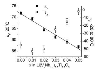
Fig. 3. Relative permittivity (filled dots) and temperature coefficient of capacitance (open dots) of  $\text{Li}(\text{Nb}_{1-x}\text{V}_x)_{0.6}\text{Ti}_{0.5}\text{O}_3$  ceramics at 1 MHz.
