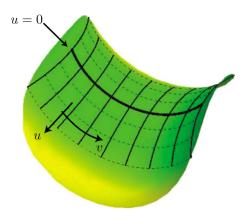
FIG. 1. (Color online) Geodesic coordinates can be constructing starting from a curve (thick line) parametrized by v, at which u =0. The geodesics perpendicular to the u=0 curve are parameterized by their arc length u (thin lines). The curves perpendicular to the geodesics (dashed lines) constitute a coordinate system in which the metric takes the form of Eq. (1).
