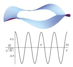
FIG. 3. (Color online) A typical minimal energy strip with four wrinkles and prescribed metric  $\rho_1$ , with  $\bar{K} = -(1/9)w^{-2}$ ,  $u_0 = (5/\pi)w$ , and t = 0.01w found by numerical minimization. Below, the mean curvature of the center line is displayed.
