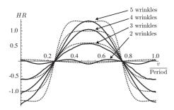
FIG. 8. The mean curvature HR along the center line of a  $\rho_1$  strip with t/w=0.006 and  $\bar{K}w^2$ =-0.029 with 5, 4, 3, and 2 wrinkles (solid) compared to theoretical predictions (dotted) along the center line.
