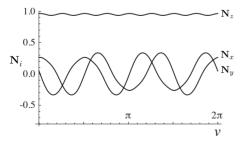
FIG. 5. The three components of the normal for the strip of Fig. 3 along the center line, which makes a nearly constant angle with the z axis. The average z component is  $\langle \mathbf{N} \cdot \hat{z} \rangle = N_z \approx 0.950$  compared to the predicted value  $\cos \phi = 0.952$ . The variance  $[\langle (\hat{N} \cdot \hat{z} - N_z)^2 \rangle]^{-1/2} \approx 0.01$ .
