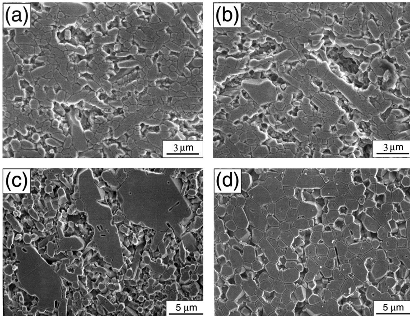
**Fig. 1.** SEM micrographs of Nd-1512 ceramics heated at (a) 25°C/min and (b) 5°C/min and of Yb-1512 ceramics heated at (c) 15°C/min and (d) 5°C/min. Micrographs correspond to Nd-25, Nd-5, Yb-15, and Yb-5 in Table I.
