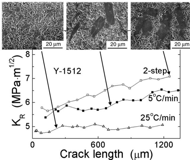
Fig. 2.  $R$ -curves and SEM micrographs of unseeded Y-1512 following three heating schedules as shown. Curves and micrographs correspond to Y-25, Y-5, and Y-2st in Table I.
