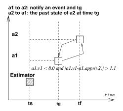
Figure 16. POSEP Synchronization stage (event notification)
