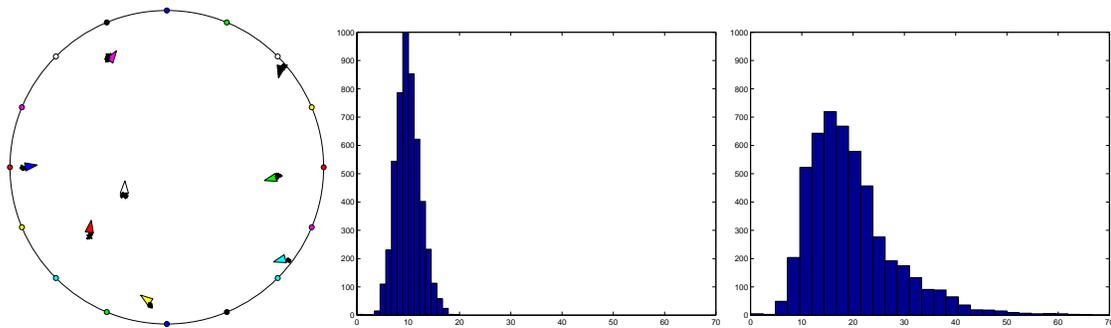
Figure 9: **Left:** Simulator snapshot showing robot positions overlaid with corresponding particle set estimates. **Center, Right:** MSE histograms for the 1.42-approximation and static assignment trials. The former reduces MSE in position by 50%.
