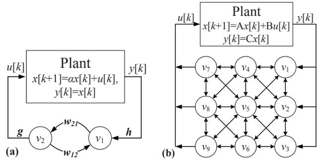
Fig. 4. Two examples of WCNs; (a) A plant with a scalar state controlled by a WCN where each node maintains a scalar state; (b) A single-input-single output plant with  $\mathbb{R}^3$  state controlled by a WCN where each node maintains a scalar state.
