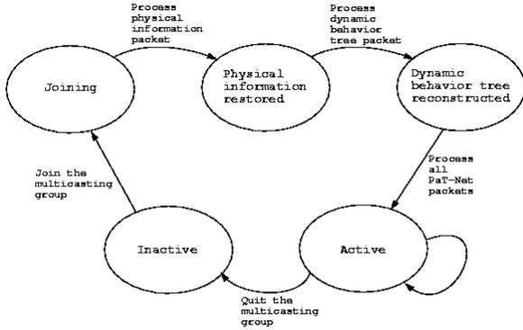
Figure 2: The life cycle of a drone LP
