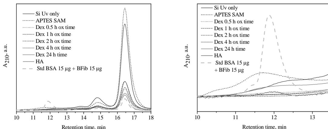
**Figure 3.** SEC of mixtures of BSA and Fg displaced from different solid substrates (for details see the text). Column and conditions as in Figure 1.
