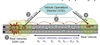
Figure 1. A hybrid simulation with real vehicles communicating across multiple simulated vehicles
