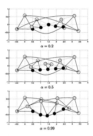
Figure 4: Three interpolating motions for a set of three planar robots as geodesics of a modified metric defined in the configuration space.
