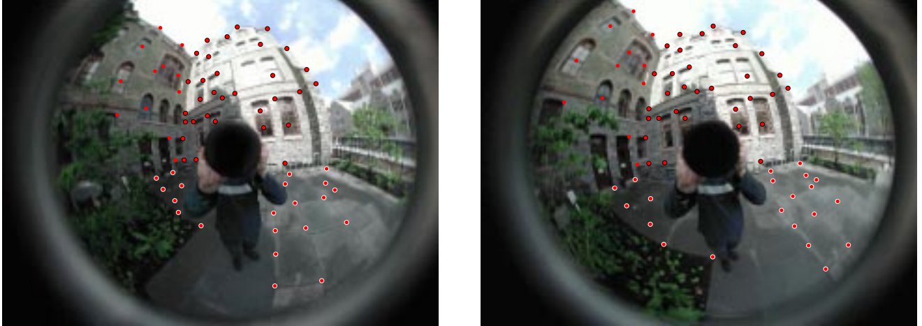
Figure 5: Two images taken with the same parabolic catadioptric camera. Points are those used for correspondence. Points highlighted in white are on the ground plane; points highlighted in black are on one side of the building facade.
