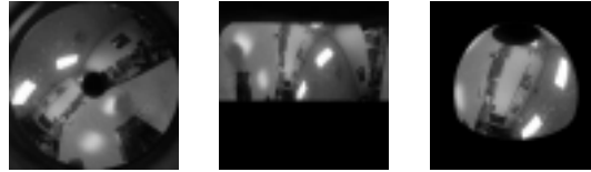
Figure 1: On the left is a parabolic catadioptric image. In the middle is the spherical image represented on the \theta - \phi plane, and on the right is the image displayed on the sphere.
