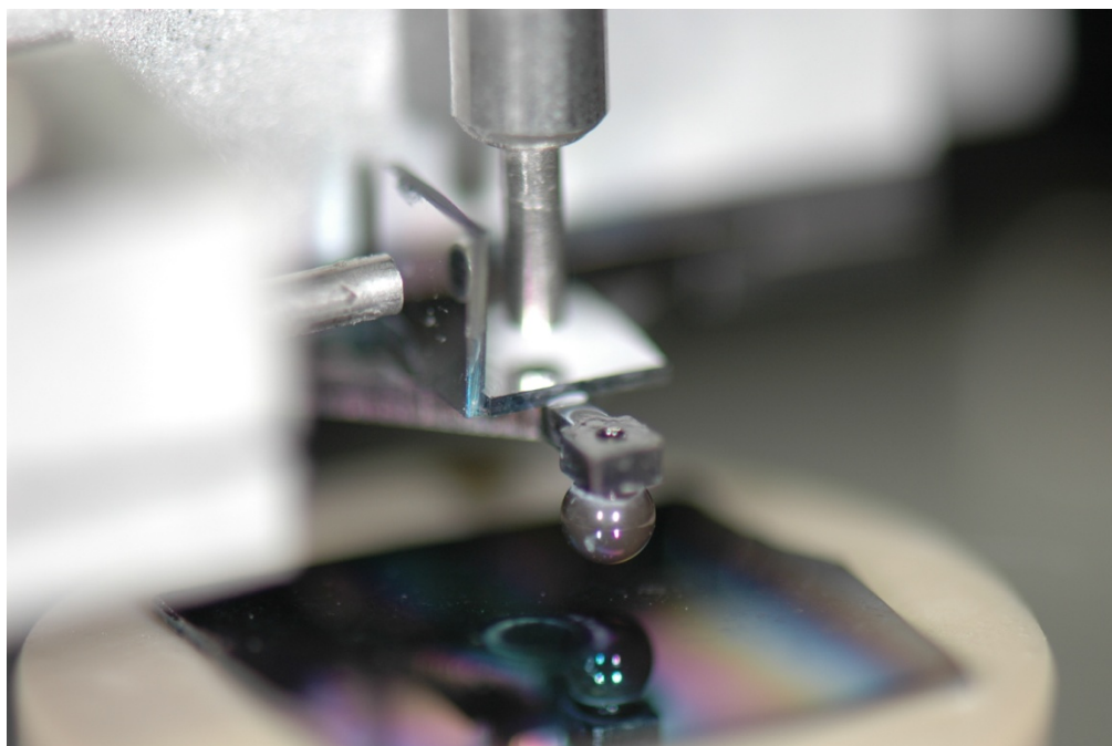
Fig. 2.6: Zoomed image showing UNCD-coated sphere and flat in tribometer.
