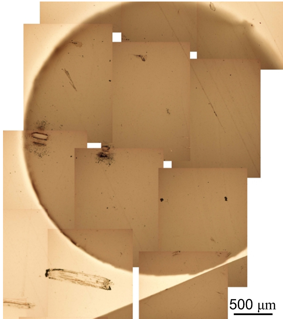
Fig. 2.17: Optical image of UNCD substrate coated with platinum (light colored areas)
