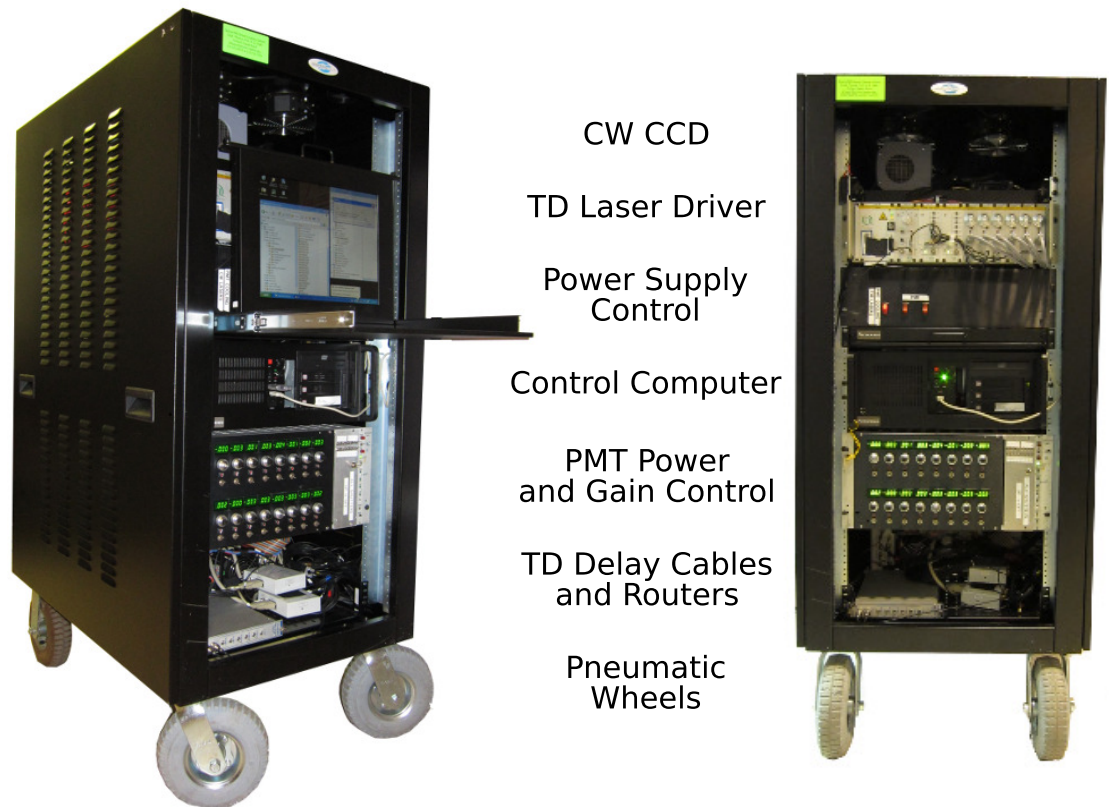
Figure 6.14: Photos of the mobile opto-electronics system for GenIII. Of special note are the CW CCD (Andor iKon, visible in upper left of right image), TD Laser Driver (Picoquant Sepia, second row in right image), Control Computer (containing the Becker and Hickl SPC-134 TCSPC cards), and shock-absorbing pneumatic wheels.
