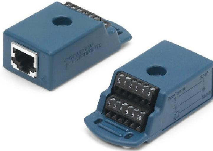
Figure A.4: NI-9949 RJ50 screw terminal adapters. Omega LCEB mini-beam load cells attach to the terminals in the following way: green wire  $\rightarrow$  2, white wire  $\rightarrow$  3, red wire  $\rightarrow$  6, black wire  $\rightarrow$  7.
