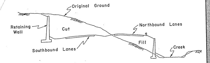
Use of retaining walls, cuts, and fills in a creek valley setting, I-476. The creek would be channelized. Planned 8' concrete sound barriers not shown. (Recall that these valleys are wooded; this is not shown in the illustration).
