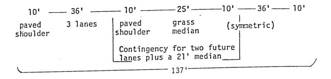
The two 10' median shoulders, together with the 25' grass median, form enough space to add two future lanes of traffic plus a 21' median (intended for median shoulders, plus a barrier).
