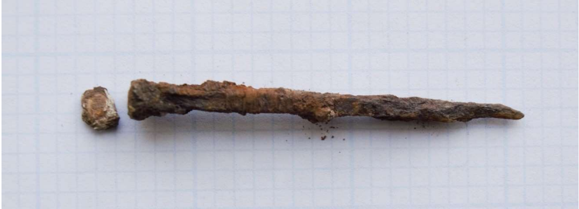
Figure 17. Nail extracted from the interior window surround of the window to the east of the front door on the north facade. Technological features indicate this is a wrought nail. Source: Author.
