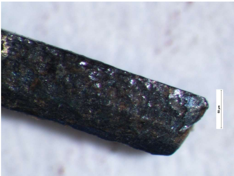
Figure 19. Cross-grain visible on a nail embedded in a piece of detached applied moulding. Magnified 10x. Source: Author.
