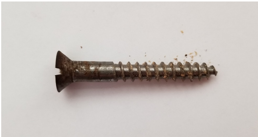
Figure 23. Screw removed from the stair baluster railing on the second floor showing machined head and gimlet point, indicating the likely manufacture date to be post 1846. Though the woodwork is likely from the 1780s campaign, the presence of modern screws supports the hypothesis that it was moved to its current location during the Raymond campaign. Source: Author.
