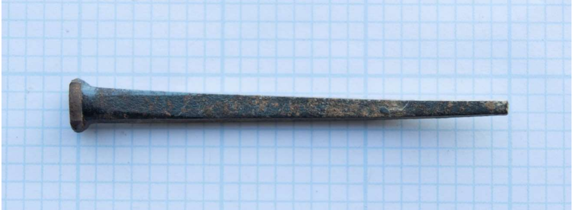
Figure 20. Cut nail extracted from the first-floor boards. Diagnostic features described by Wells indicate this nail was likely produced between 1820-1890. Source: Author.
