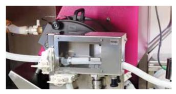
Figure 6. The Automated Pressure Control Valve (PCV) features a clear outer door enabling a clear view during operation. If the door is opened during operation, the valve automatically shuts off ensuring operator safety.
