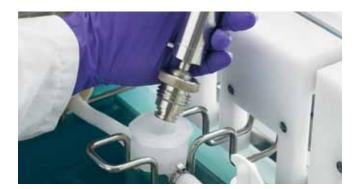
Figure 4. The innovative low dead volume t-connector prevents pressure sensor contact with the fluid path.
