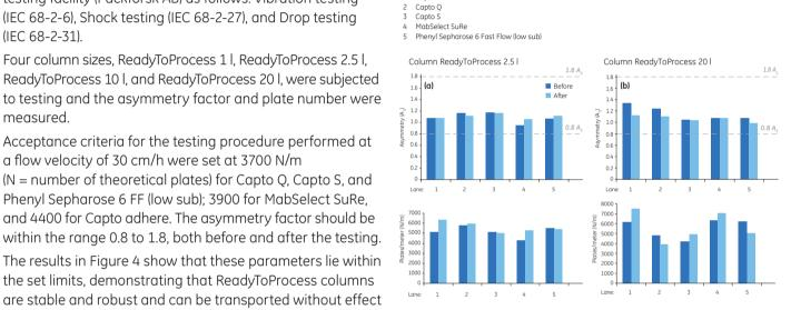
Fig 4. Transport simulation studies on ReadyToProcess 2.5 I (a) and ReadyToProcess 20 I (b) columns show that both the number of theoretical plates, N/m, and the Asymmetry factor, A<sub>s</sub>, were within the predefined ranges after testing.
