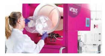
Figure 3. A pivoting retentate recycle tank design facilitates container loading.
