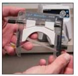
1. Select tubing, load tubing into cartridge, and set tubing retainers.
