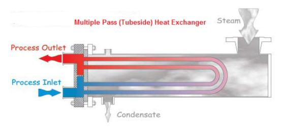
Heat exchanger designs vary based on throughput, thermal duty, local maintenance requirements, size requirements, heat transfer media, the chemical state of the materials (liquid or gas) and physical properties of the materials (e.g. specific heat, viscosity, specific gravity, fouling factors, etc.). Each design incorporates all of these factors. After looking at heat transfer requirements, the designer takes the following into consideration:
