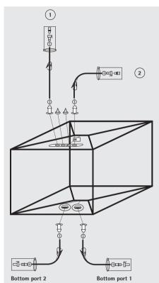
Standard Flexel® 3D bags with silicone tubes (100 L to 500 L) Standard Flexel® 3D bags with silicone tubes (1,000 L)
