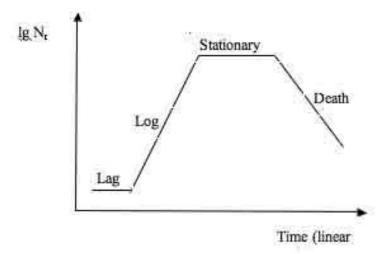
Figure A.1. Cell growth curve consisting of four distinct phases, lag, log, stationary, and death. The log of the number of cells or cell concentration(y-axis) is plotted against linear time (x-axis). This basic model of cell growth holds true for most cell types. From Börje Lindström, LTU, Sweden
