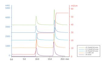
**Fig 5.** Stacked chromatogram comparing step elution on the five different columns. The elution buffers were 50 mM sodium acetate, 0.3 M NaCl, pH 5.0 and 50 mM sodium acetate, 0.65 M NaCl, pH 5.0. The elution steps were 3 CV each. The chromatograms were obtained using ÄKTAready system, except for XK 16/40 which was run on an ÄKTAexplorer™ system.
