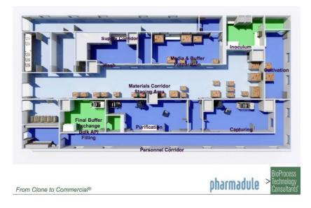
Figure 10.2 Design schematic for single-use influenza vaccine manufacturing facility with insect cell culture
