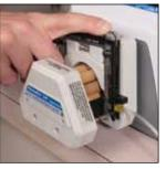
2. Snap cartridge into place on pump head.
