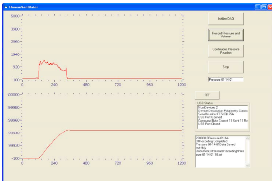
Figure A.8. Representative read-out of real-time inspiratory flow rate and volume acquired with the MRI-compatible pneumotachometer.
