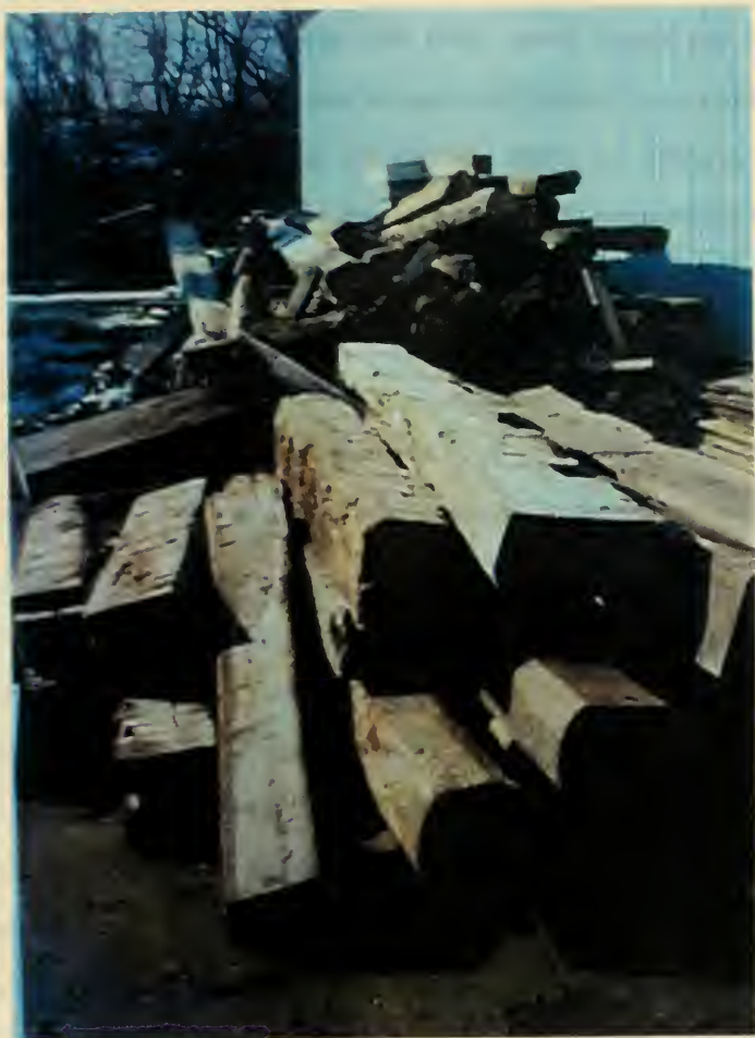
Figure 4. Salvaged floor joists and roof rafters from demolished industrial buildings before being milled at Sylvan Brandt's workshop and warehouse. (Photo taken by author, February 2001.)
