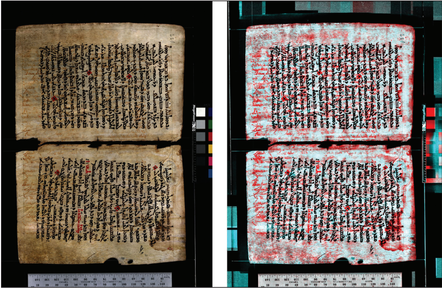
FIGURE 1. Visual appearance of bifolio 214v–221r on the left and the pseudocolor rendering generated from the ultraviolet ( \lambda = 365\text{ nm} ) and a near-infrared band ( \lambda = 780\text{ nm} ) on the right.
