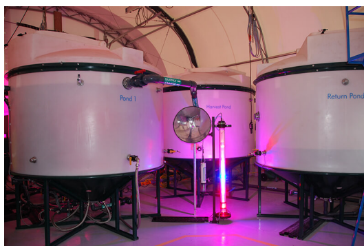
Figure 4.3: Pond Technologies’ internally illuminated 1000L tank photobioreactors.
