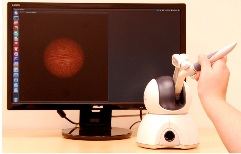
Figure A.3: A person using a Phantom Omni to interact with the cork texture on a virtual sphere.
