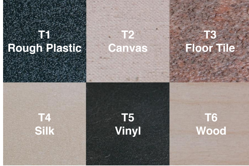
Figure 2.3: Six textures that were haptically modeled with the presented methods. These materials were chosen to provide a set of textures that was diverse in roughness, hardness, slipperiness, and fineness of surface features.
