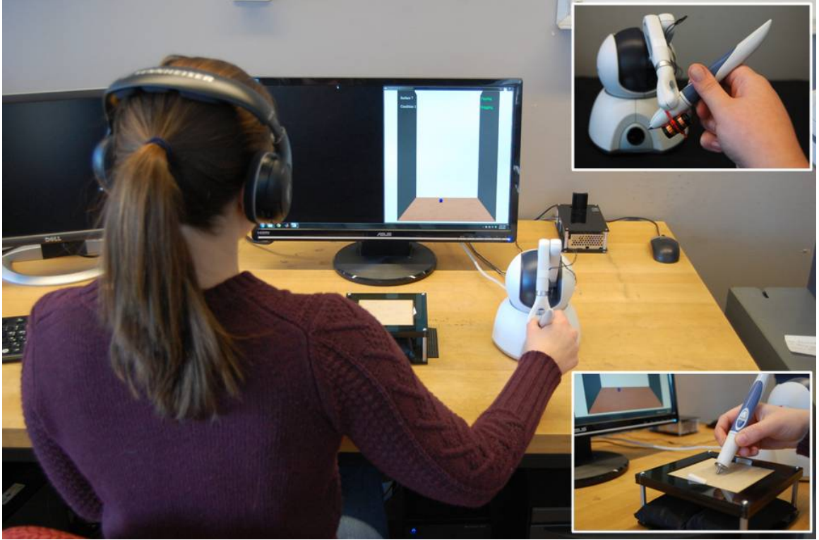
Figure 4.8: Experimental set-up. The subject sat at a table in front of a computer and wore headphones playing pink noise to mask auditory cues. The subject used an Omni to feel the virtual surfaces and an adapted Omni handle to feel the real surfaces.
