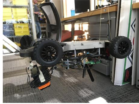
Fig. 10: Test setup of the vehicle.
