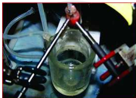
Fig. 2. Simultaneous fluorescence-phosphorescence measurements on a rat heart (upper center)
