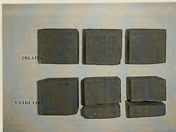
Figure 6.8: Untreated and treated stones after wet-dry cycling test The untreated stone (#3) that had pre-existing cracks before being tested broke while the treated stone (#3) could resist the damage caused by wet-dry cycling. The untreated stone (#2) broke after the test although the pre-existing damage did not perform.
