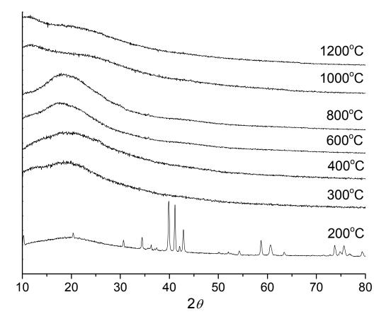
**Supplement 3.** X-ray diffraction (XRD) spectra of CDC produced at different temperatures (Cu  $K_{\alpha}$  radiation).
