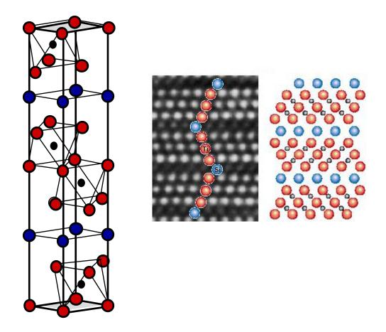
**Supplement 1.** Unit cell of  $Ti_3SiC_2$ , high-resolution TEM image of  $Ti_3SiC_2$  along [110] zone and a schematic of (110) plane. Ti atoms are shown in red, silicon in blue and carbon in black.
