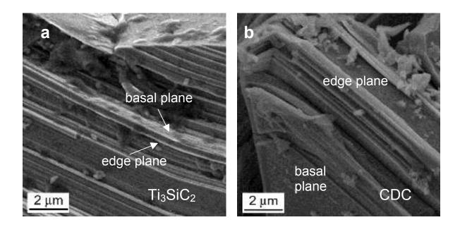
**Fig. 4.** SEM micrographs of a sample surface **a**, before and **b**, after chlorination at 300°C. Lamellar structure of  $Ti_3SiC_2$  is clearly seen and it does not change after metal extraction. The sample in (B) is fully amorphous, but maintains the lamellar structure of the carbide. No change in the surface quality or grain morphology occurred after conversion of carbide to carbon.
