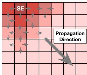
Figure 2: Cardiac tissue is modeled as a 2D grid of cells. *SE* is a self-exciting cell. After *SE* depolarizes, the neighboring cells depolarize as well. The delay in propagation is determined by the velocity of depolarization, how long the cell remains depolarized, the resistance to current flow between cells, and the current state of the neighboring cell. The chain reaction of depolarization causes an aggregate wave of AP propagation.
