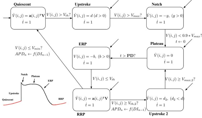
Figure 5: Hybrid model of one hybrid cellular automaton. AP figure from [8].  $V_{th,2} > V_{th}$ ,  $V_{max,2} < V_{max}$ .  $DI_n$  is the Diastolic Interval of  $n^{th}$  beat, and  $f$  is the restitution function which determines the APD for the subsequent cycle based on the DI of the current cycle.
