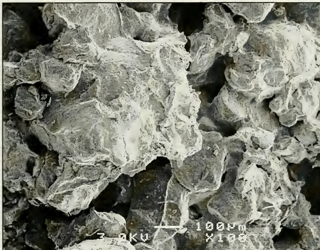
Figure 31. Butterbaugh amended adobe, 25% E-330, 100x magnification. This sample was taken from an adobe brick made by Darrell Butterbaugh in 1975 and placed on the roof of the University Museum in Philadelphia that year. Made from an obviously sandy soil, the adobe is still intact. Compare the soil texture with Figure 32 , a Mesa Verde amended mortar. Both images are 100x magnification. White bar is 100 µm.
