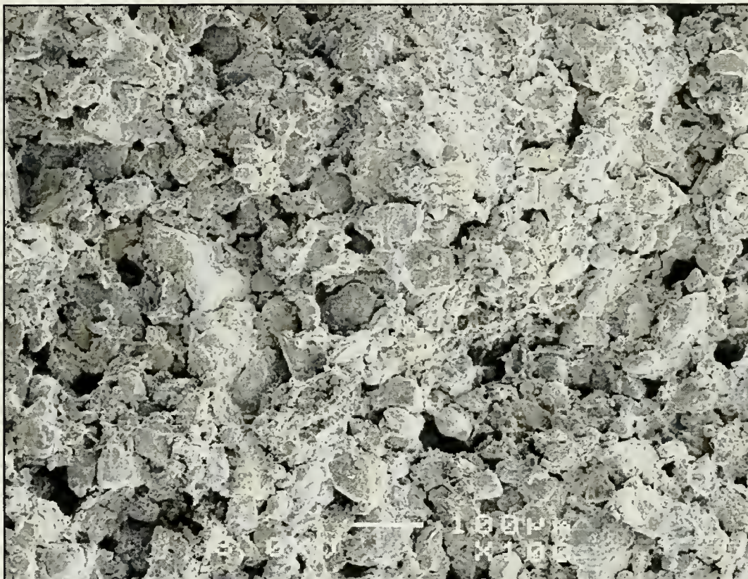
Figure 32. Coyote Village amended mortar, Mesa Verde, 100x magnification. This amended earthen mortar sample (between 25% and 33% E-330) was taken from a deteriorated mortar location at Coyote Village, near Far View Ruin, on Chapin Mesa. Compare the texture of this soil with the sandy modified adobe sample in Figure 31 . White bar is 100 \mu\text{m} .
