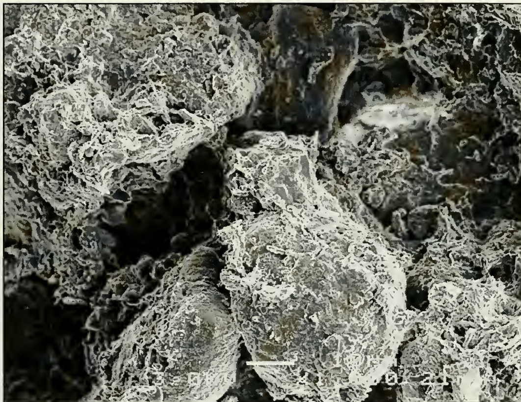
Figure 21. Mesa Verde Blend earthen mortar, 0% E-330, 1,000x magnification. In this sample of unamended Mesa Verde Blend earthen mortar, the soil particles stand out in sharp relief. Compare with the amended Mesa Verde Blend earthen mortar, Figure 22 . White bar is 10 \mu m.
