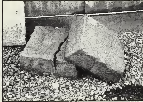
Figure 5. Placed on the University Museum roof in Philadelphia in 1975, these E-330 amended adobe bricks made by Darrell Butterbaugh were still in sound condition in 1995. Although a particle size analysis of the soil was unavailable, the soil appeared to have a high sand content. A quarter is shown for scale.
