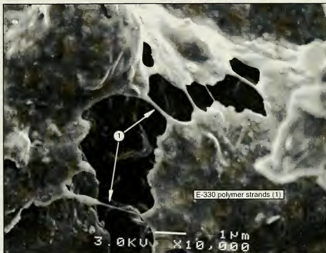
Figure 25. Far View Ruin amended earthen mortar, Mesa Verde, 10,000x magnification. This sample was taken from a dry, intact, piece of amended mortar (between 25% and 33% E-330) at Far View Ruin, on the top of Chapin Mesa. The same distinctive polymer strands seen in the laboratory samples made with Mesa Verde Blend also are visible here. Another view of the sound Far View amended earthen mortar is shown in Figure 26 . White bar is 1 \mu\text{m} .
