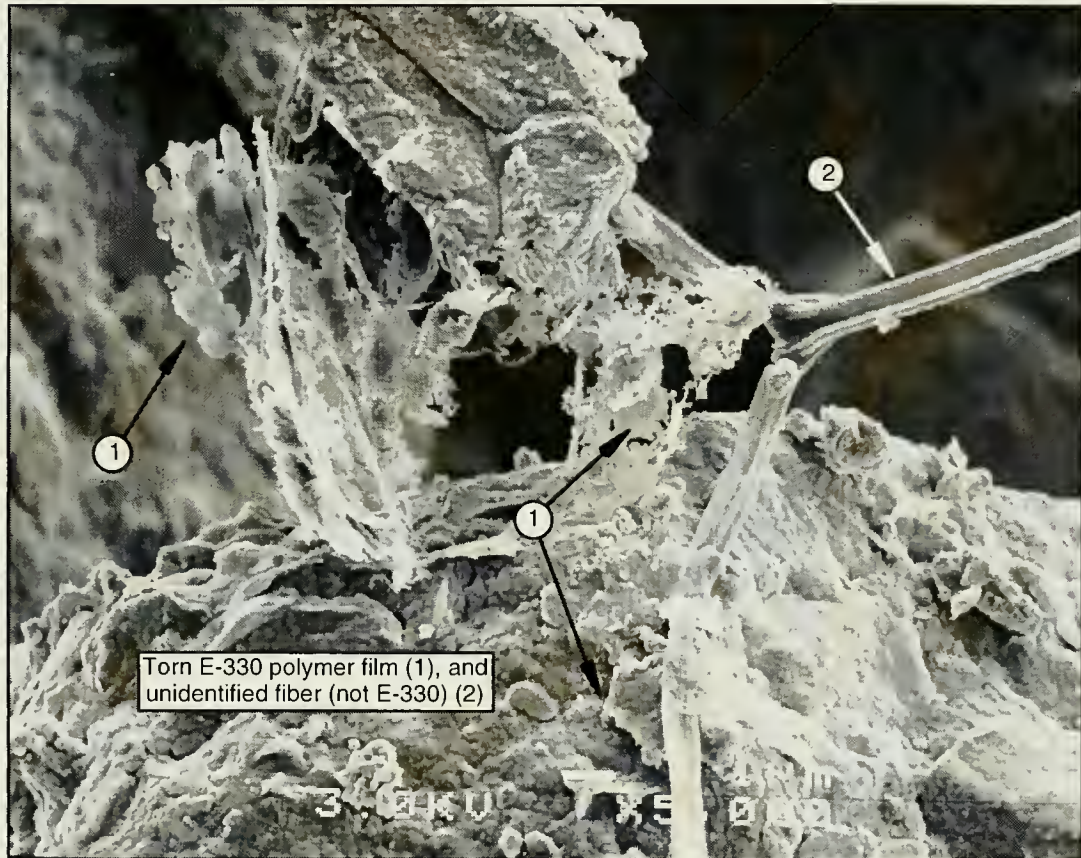
Figure 34. Long House Ruin amended earthen mortar, Mesa Verde, 5,000x magnification This deteriorated amended mortar was sampled from Long House, a cliff dwelling on Wetherill Mesa. The mortar there has a larger proportion of crusher fines, a sandier mix than that used on the mesa tops. Still, the mortar exhibited the flaking characteristic of Mesa Verde amended mortars. The damaged E-330 film is visible in the microphotograph. (The mortar contains between 25% and 33% E-330.) White bar is 1 \mu m.
