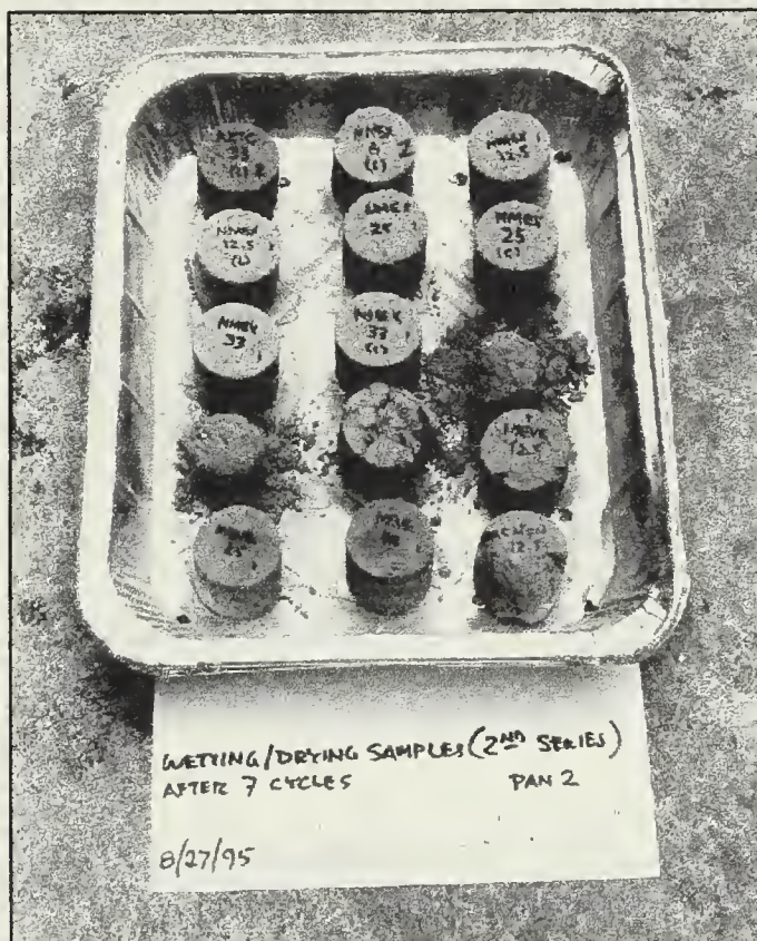
Figure 16. The wetting/drying test was the most challenging of the mortar tests. The samples were alternately soaked for five hours in room temperature water, and then dried in a warm oven, one cycle per day. The badly deteriorated samples in this tray are 6% Mesa Verde Blend earthen mortars, after 7 cycles.
