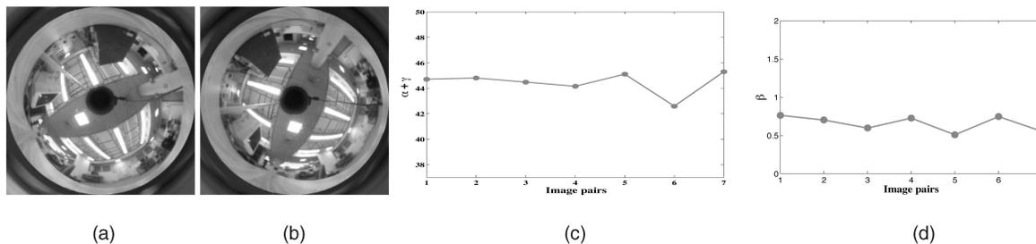
Fig. 5. (a) and (b) One of seven sequential pairs of images tested. The ground truth rotation was observed to lie at approximately  $45^\circ$  about the  $Z$  axis for each pair. (c) The estimated rotation about the  $Z$  axis ( $\alpha + \gamma$ ). (d) The estimated rotation about the  $Y$  axis ( $\beta$ ). Our algorithm correctly finds the rotation about the  $Z$  axis as well as finding only a negligible rotation about the  $Y$  axis.
