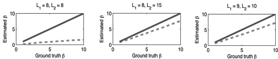
Fig. 4. Representative plots depicting the rotations minimizing the residual error in different ranges of SFT coefficients. The solid line on the diagonal marks the position of the true rotation, while the dashed line marks the rotation minimizing the residual error. Due to signal corruption,  $\beta$  will be underestimated even for small rotations.
