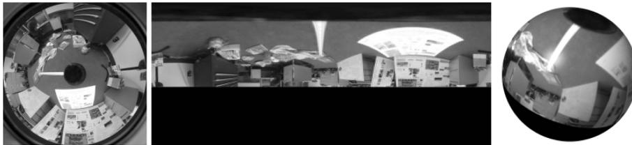
Fig. 1. Left: A parabolic catadioptric image. Middle: The corresponding spherical image on a uniformly sampled spherical grid. Right: The spherical image as it would appear on the surface of the sphere.
