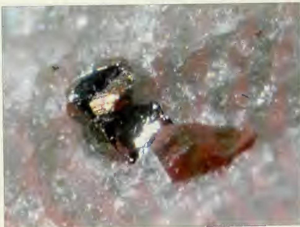
Figure 4.13: Pyrite (left) and phlogopite (right) in a fractured surface of sample 1 seen under a stereomicroscope. 38x magnification, fiber-optic illumination.
