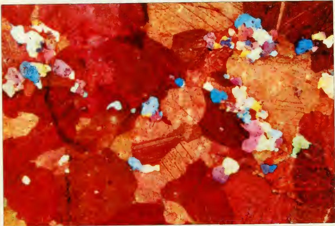
**Figure 4.41:** Crystalline calcite grains (red and orange) and silica inclusions (blue, purple, white, yellow). The silica occurs occasionally in the Cherokee marble. An unusually dense concentration is seen here. The silica forms both along the grain boundaries and within the calcite grains. 1.25x magnification, cross-polarized light, stained for calcite.
