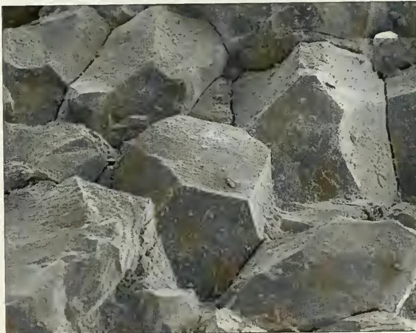
Figure 4.51: Distinct calcite crystals on a fractured Sheffield surface from sample 37. Fine cleavage planes can be seen between grains. 100x magnification, JEOL 6300FV Field Emission HRSEM.
