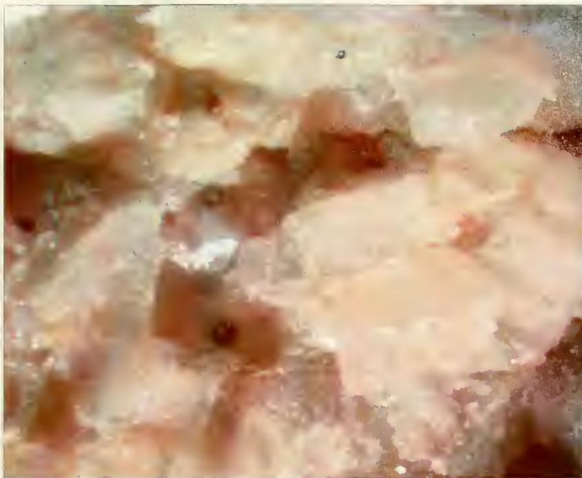
**Figure 4.22:** A fractured surface of sample 1. Intergranular cracking is more common in the weathered sample than in the fresh sample. Brown flecks of phlogopite are visible in the cracks. 7.5x magnification, fiber-optic illumination.
