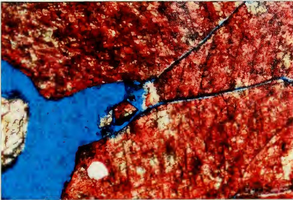
Figure 4.37: A surface grain detaching from the substrate on slide S-36. Thermally-induced deformation causes surface grains to fall off, opening microcracks that facilitate moisture penetration. 10x magnification, plane polarized light, stained for calcite.
