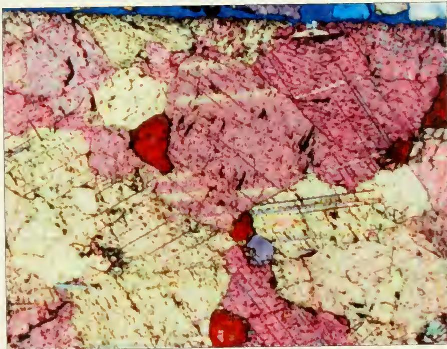
**Figure 4.6:** An absence of microcracking is evident in this photomicrograph of slide T-8. Vacuum impregnation with blue dye did not reveal any fractures. The clean surface is seen in the upper portion of the photomicrograph bordered by the blue dye. Close-up of 5x magnification, cross-polarized light.
