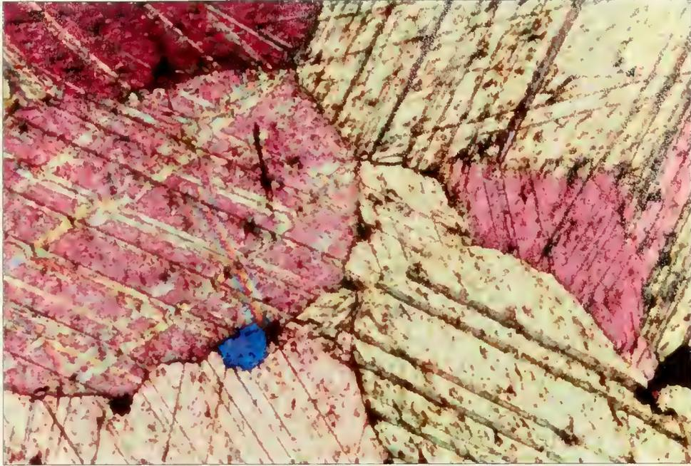
**Figure 4.42:** Highly crystalline calcite grains in slide G-26. Note highly angular, fused grain boundaries. A siliceous inclusion, seen in blue occurs along the grain boundary towards the bottom of the photomicrograph. Twinning of calcite is also seen. 50x magnification, cross-polarized light, unstained for calcite.
