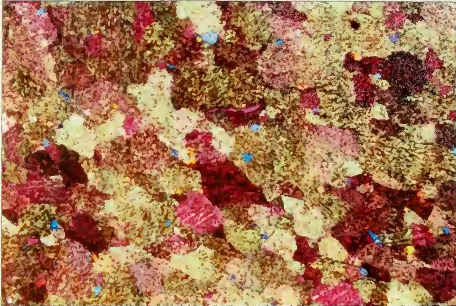
**Figure 4.25:** Typical view of fresh Sheffield grains from slide S-38 in cross-polarized light. Calcite is seen throughout, and silica is seen distributed regularly in blue and orange. 1.25x magnification, unstained for calcite.
