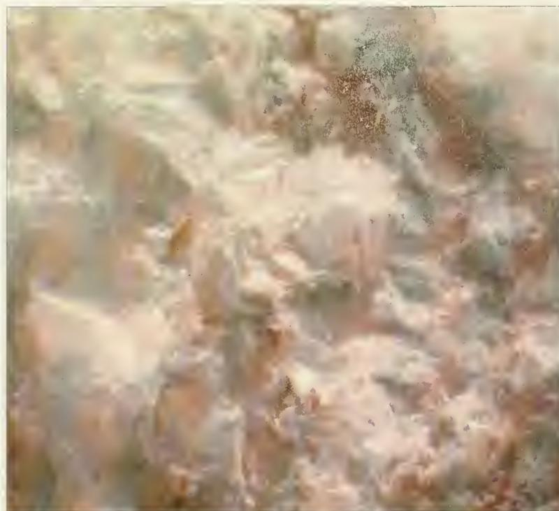
**Figure 4.7:** A fractured Tuckahoe surface from sample 8 seen in raking light. Intragranular cracking is more common than intergranular cracking. 7.5x magnification, fiber-optic illumination.
