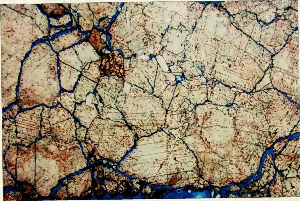
Figure 4.14: Slide T-1A, a typical weathered specimen with extensive microcracking. Crack networks are highlighted by vacuum-impregnated blue dye. Oblong phlogopite inclusions are visible at the center of the image. The exposed weathered surface is at the bottom of the picture. Photomicrograph is 1 cm wide, slide is unstained for calcite. 1.25x magnification, plane-polarized light.
