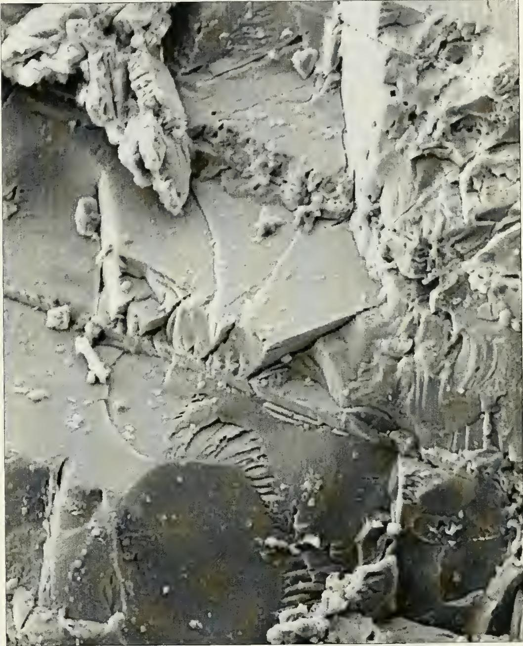
**Figure 4.49:** A fresh fractured Tuckahoe surface from sample 1. Jagged intragranular cleavage is seen to the right and top of the image and straight intergranular cleavage is seen in the center. 100x magnification, JEOL 6400 Analytical SEM.
