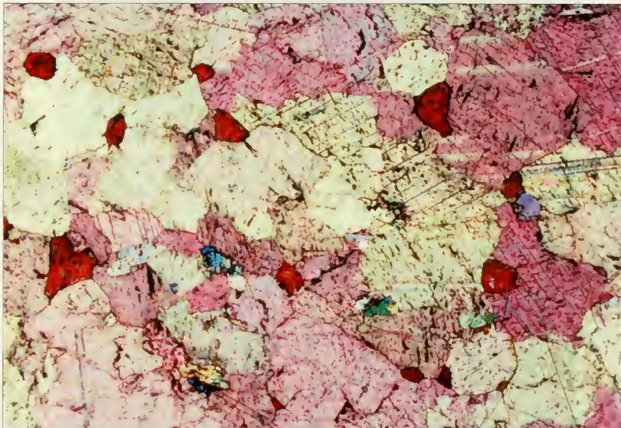
**Figure 4.2:** A typical view of fresh Tuckahoe marble from thin section slide T-8. Red stained calcite is interspersed with dolomite. The structure appears uniform and crystalline at the top of the photomicrograph. In the lower left, the structure appears more conglomerated. 5x magnification, cross-polarized light.
