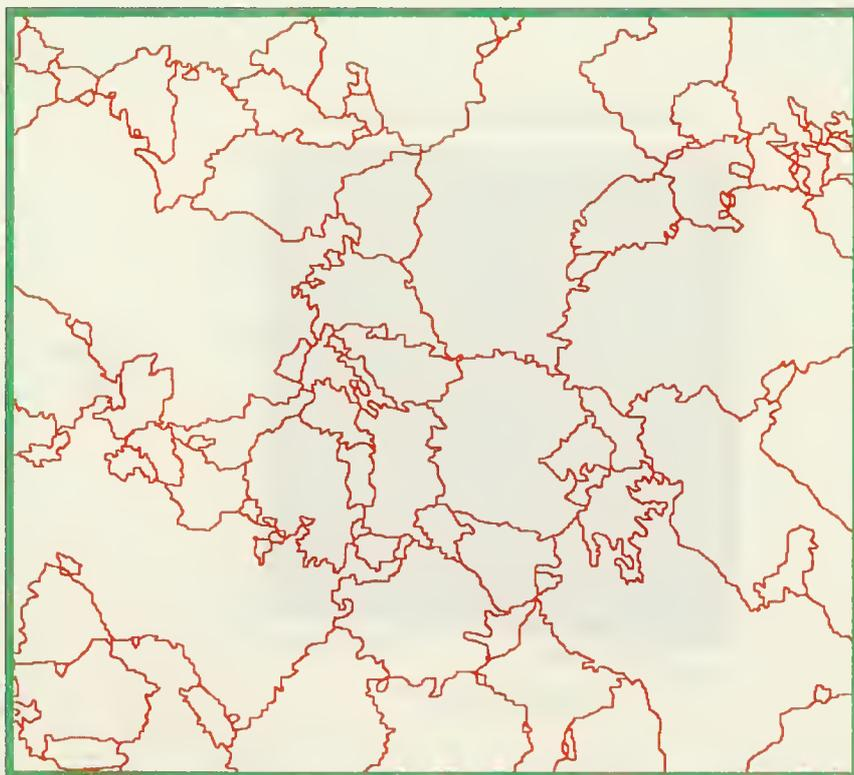
**Figure 4.23:** Digitized grain boundary image of 1 square cm of Tuckahoe slide T-1B.
