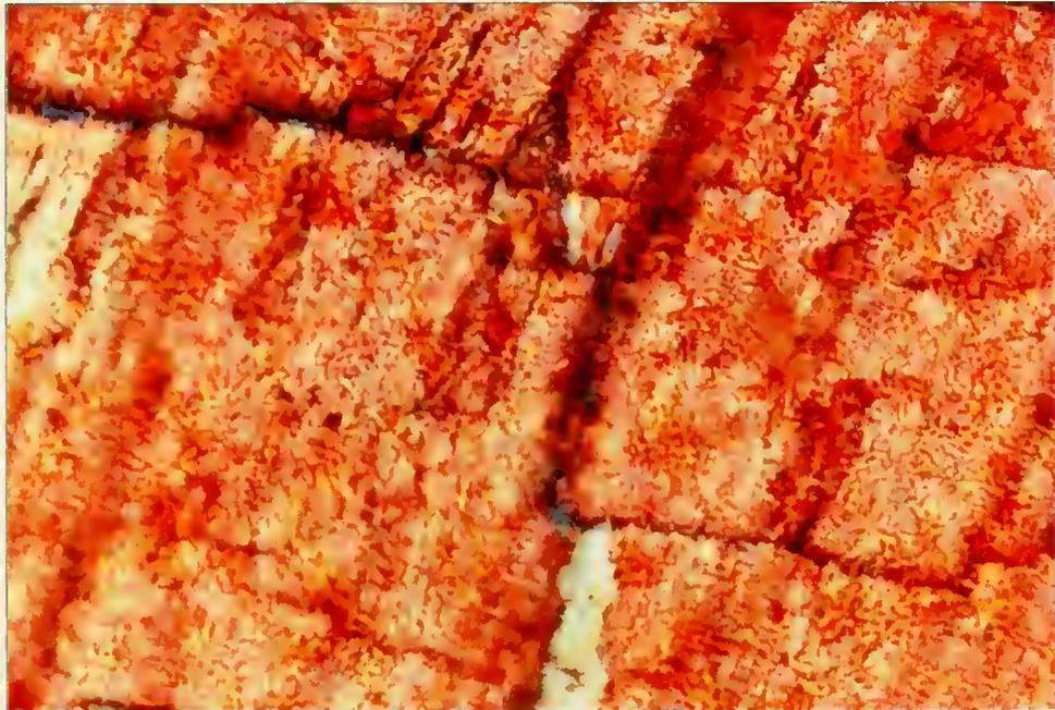
**Figure 4.43:** Microcracking in fresh Cherokee slide G-29 seen at high magnification. Fractures follow the rhombohedral mineralogical structure of calcite. 40x magnification, plane-polarized light, stained for calcite.
