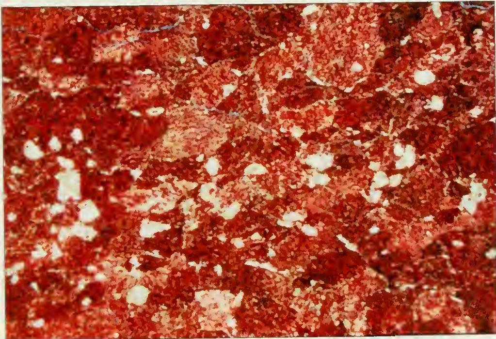
Figure 4.32: Silica inclusions sometimes appear in bands. Here they are gathered in the center and bottom of the slide, S-36. 1.25x magnification, plane-polarized light, stained for calcite.
