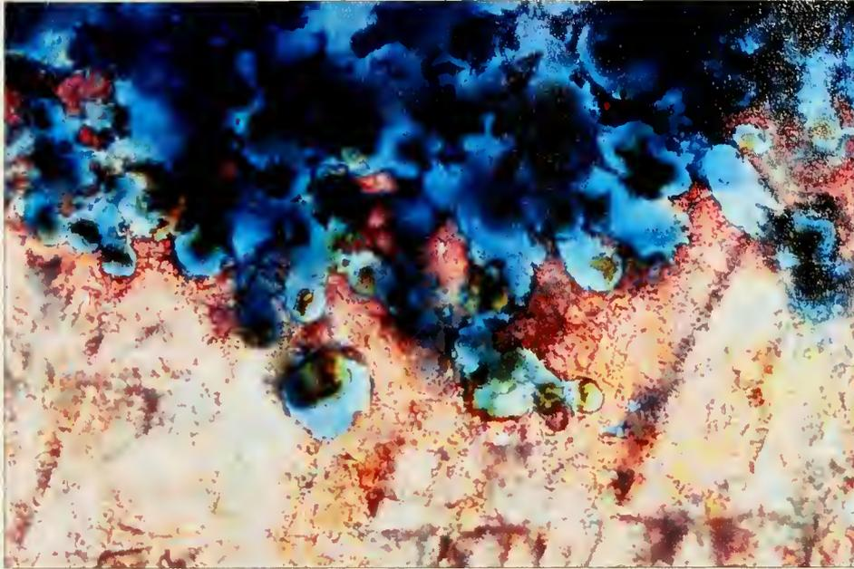
**Figure 4.39:** Biological growth on the surface of the quarry sample, slide S-15. Fungi have digested the first 2 mm of the surface, creating a porous substrate. 20x magnification, plane-polarized light, stained for calcite.
