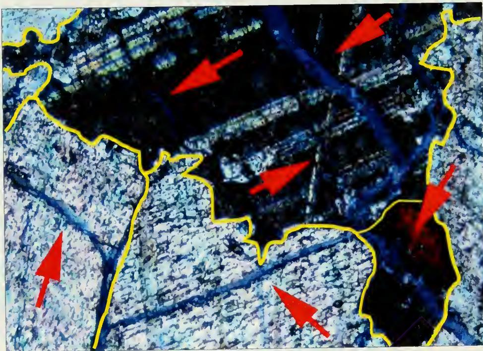
Figure 4.15: Intragranular cracking below a weathered surface in thin section slide T-1B, taken from an abacus on the North Portico. The original grain boundary is shown in yellow, cracks are indicated by the presence of blue dye, and intragranular cracks are indicated by red arrows. 50x magnification, cross-polarized light.
