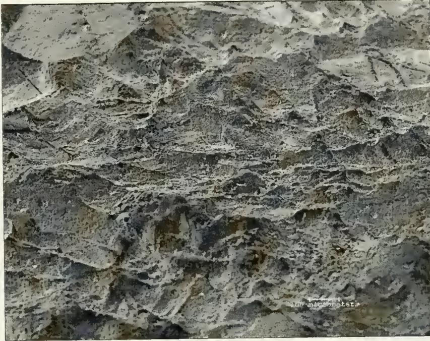
**Figure 4.52:** Etching of calcite grains on a weathered Sheffield surface from sample 36. Note the outline of an individual calcite crystal in the upper left hand of the image. 100x, JEOL 6300FV Field Emission HRSEM.
