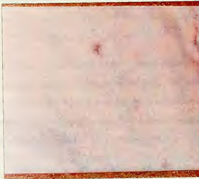
**Figure 4.47:** A block of Georgia Cherokee marble at the NIST Stone Exposure Test Wall in Gaithersburg, MD. After 50 years of outdoor exposure, the Cherokee block shows surface decay of less than a few microns. No staining from pollution was observed. The block is 2 ft. tall.
