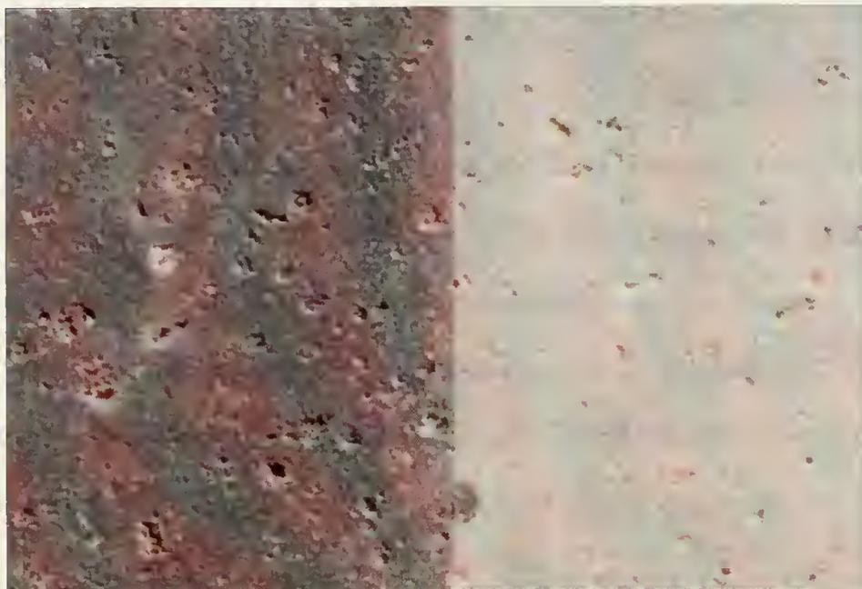
Figure 3.4: Close-up of cleaning test number 10. Gray discoloration and pock-marking are evident.
