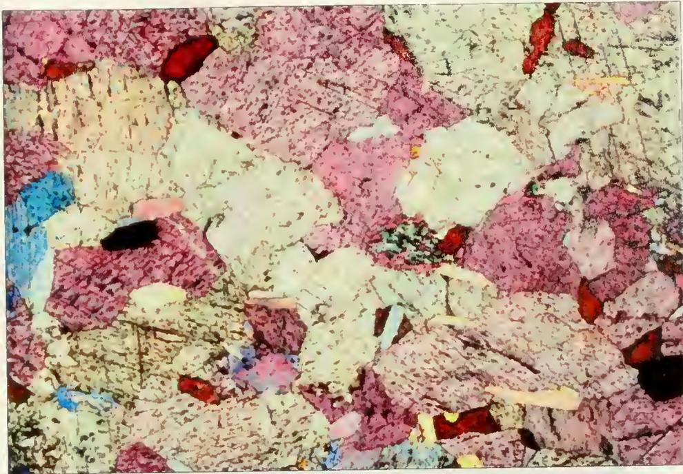
**Figure 4.5:** Numerous inclusions are seen in the lower half of the picture. The green inclusion appears to be tremolite, while the numerous oblong inclusions are phlogopite. The variety of minerals creates a heterogeneous structure. 5x magnification, cross-polarized light.
