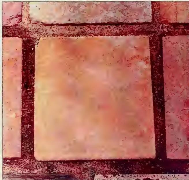
**Figure 3.12: An iron-stained sample of Lee marble in the Stone Exposure Test Wall at the NIST. Like the Tuckahoe sample, discoloration due to pollution was not noticed.**
