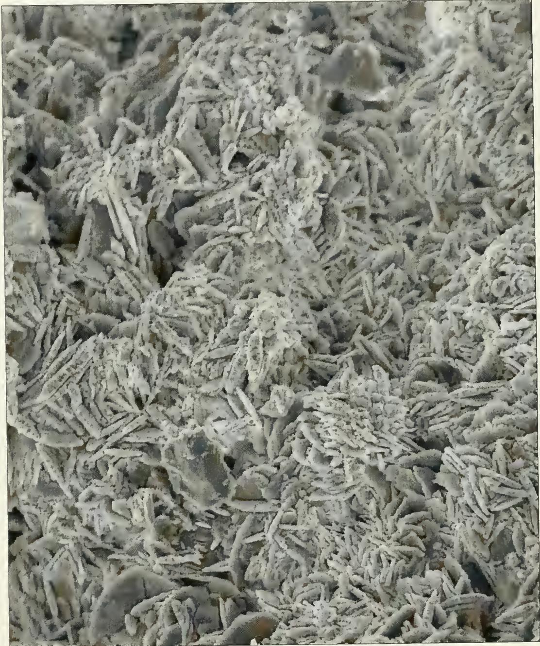
Figure 4.48: Gypsum encrusted surface of sample 1. 100x magnification, JEOL 6400 Analytical SEM.
