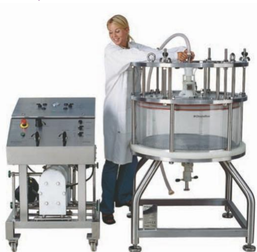
Fig 3. Packing Chromaflow columns with the dedicated packing station is convenient and simple.
