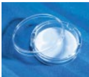
3419 75mm Polycarbonate Transwell Insert
