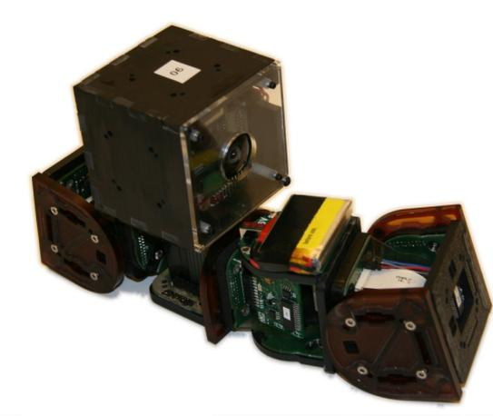
Figure 7.1: Each cluster in the modular robot is composed of four CKBot modules and a smart camera system.
