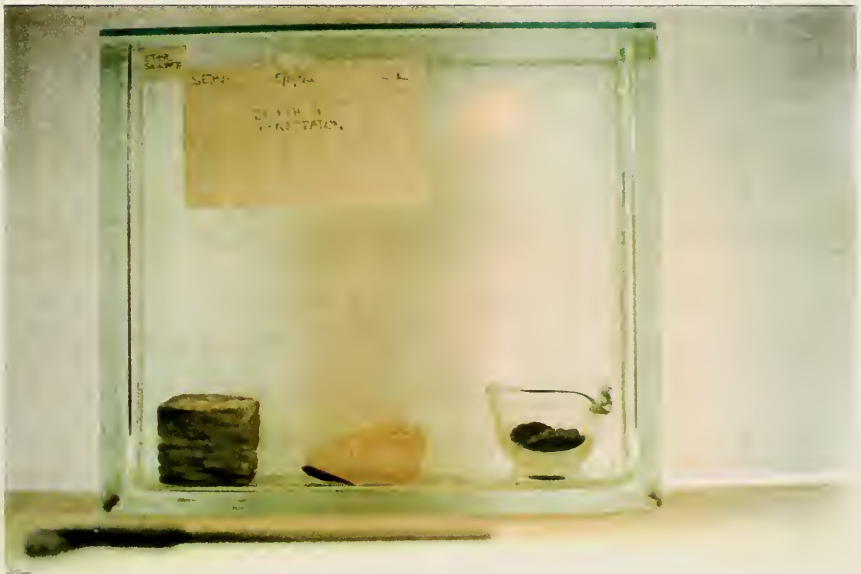
Figure 11. Samples during testing of consolidant penetration depth.
