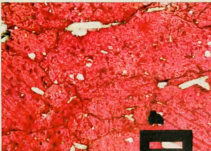
Figure 6. Thin Section of Sample III, crossed polars, 100X, stained for calcite. Note graphite inclusion, replacement within calcite matrix.
