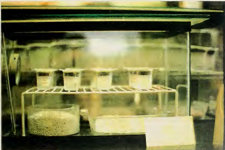
Figure 16. Samples during water vapor transmission rate testing.
